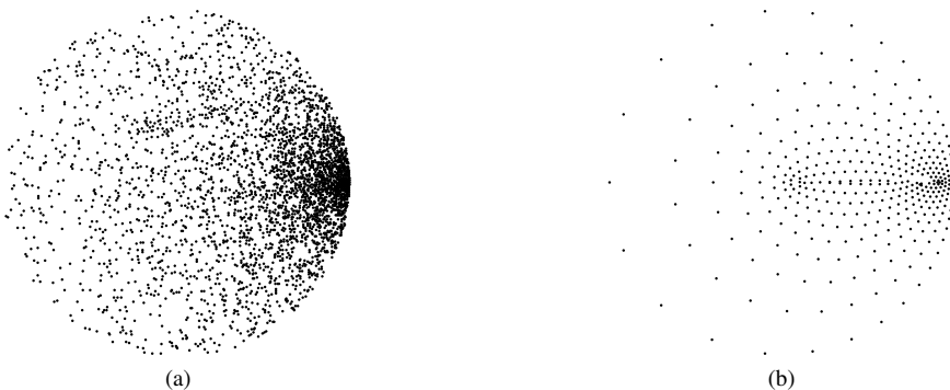
Figure 1: Node placement in the unit disc using: The rejection method, (a) and our algorithm, (b) with h(x, y) = 0.2\sqrt{(x-1)^2 + y^2} + 0.04 .
