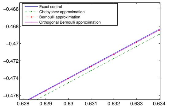
**Figure 12.** Control of the 3rd iteration by algorithm 1 and 2 compared with the exact control and control of method 3 for example 3.
